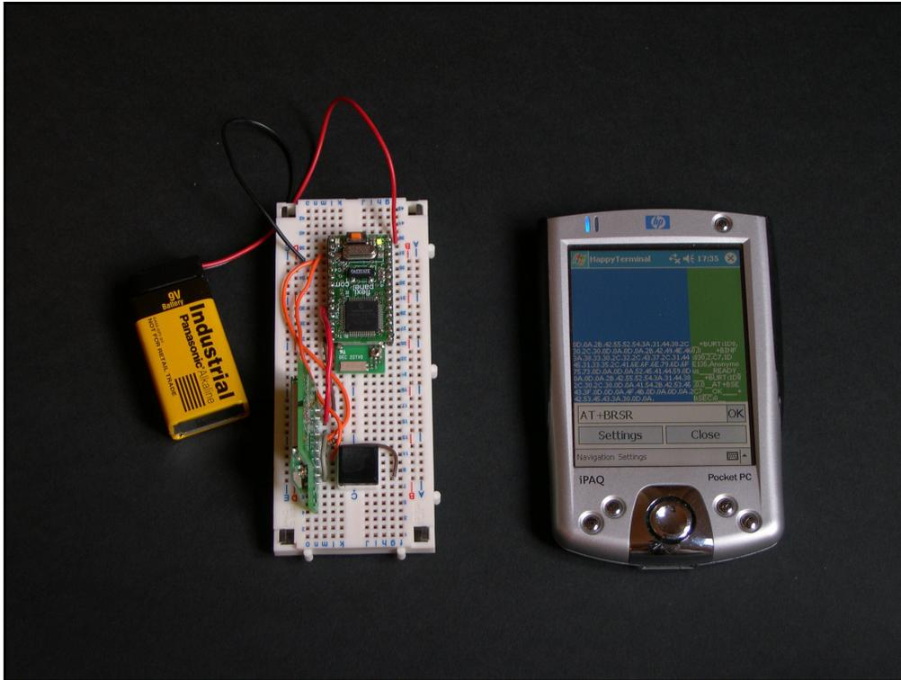
*Figure 2. The ToothPIC terminal emulator (top) with serial connection to a microcontroller module under test (bottom). The serial terminal is ‘emulated’ on a Pocket PC or Windows PC using the Bluetooth link.*
