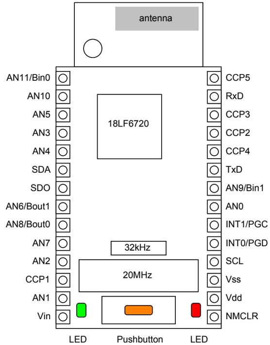
Figure 1. Pinout of the ToothPIC module. The FCC certified Bluetooth radio and the voltage regulator are mounted on the underside of the board.
