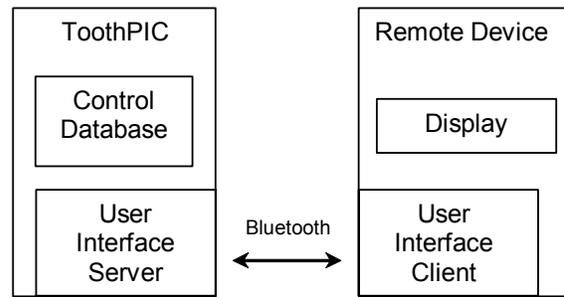
*Figure 3. The user interface is managed by a server on the ToothPIC and displayed by a client such as a Pocket PC or Windows PC.*
