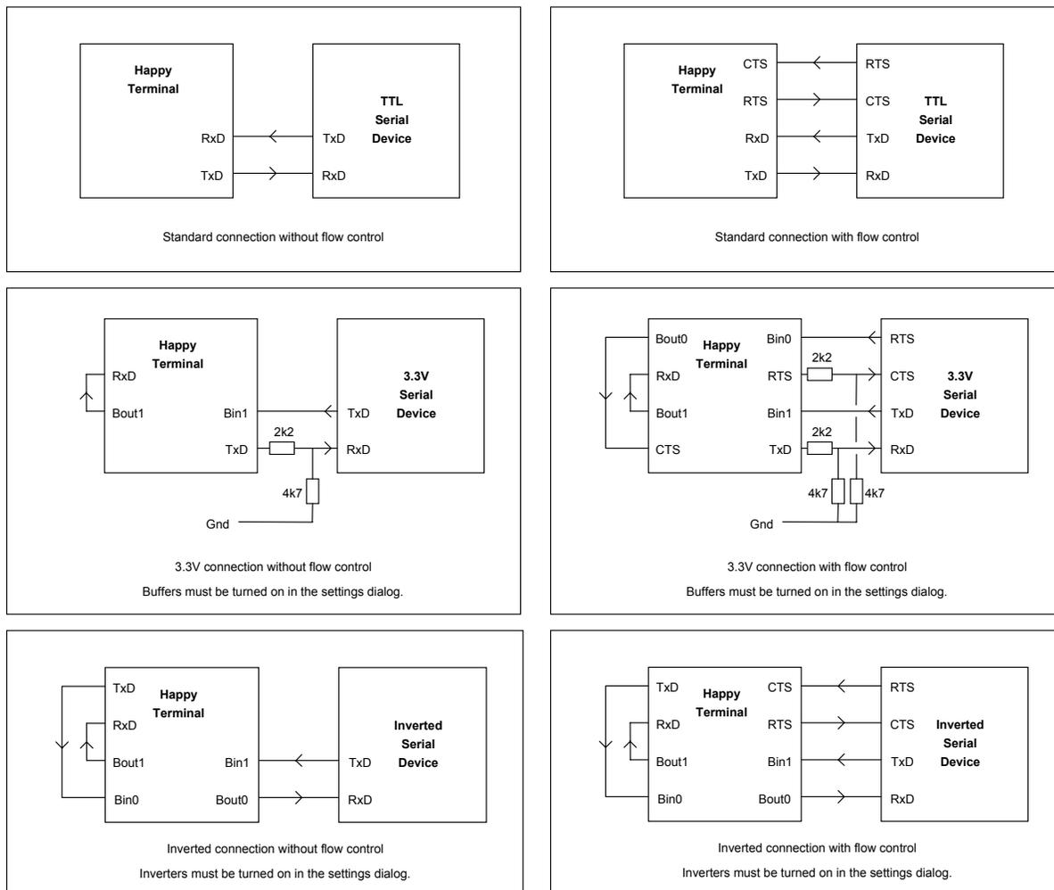
Figure 7. Various pin configurations for the terminal emulator.
